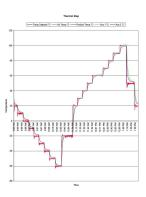
NOTE: I.MX6 devices have a built-in failsafe that will shut system down gracefully if CPU temp reaches 101°C. Failsafe performed as expected and system recovered as soon as CPU temps were lowered back to less than 100°C. If customer has an application that requires greater than 100°C we will have to bypass failsafe and further HALT testing is recommended.
