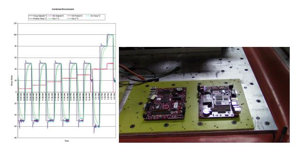
NOTE: 5603 lost communication with each transition from cold to hot. It performed fine when just facing one variable, but the transition impacted it unexpectedly. It also did not display these symptoms during just temperature thermal transition, just in combined environment. Device would recover without assistance or interference. The second unit did not display same characteristics and handled transition smoothly.
