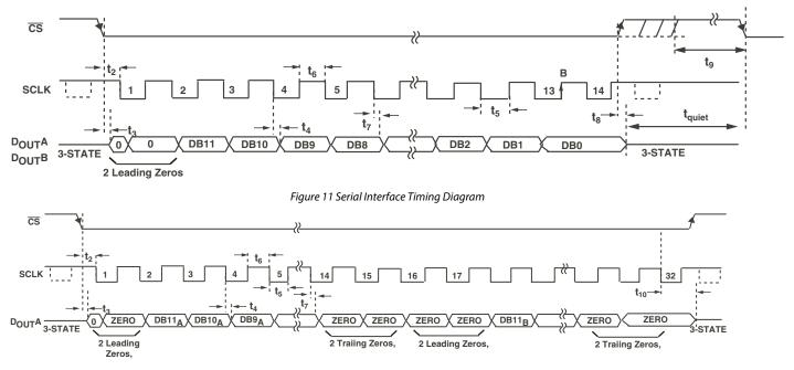
Figure 12. Reading data from Both ADCs on One Dout Line with 32 SCLKs
