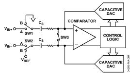
Figure 4. ADC Conversion Phase
