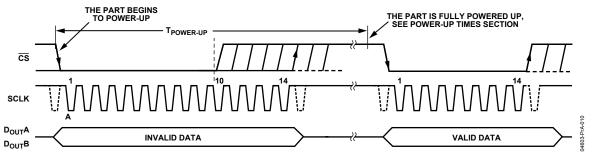
Figure 10. Exiting Partial Power-Down Mode
