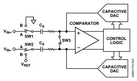
Figure 3. ADC Acquisition Phase
