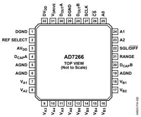
Figure 2. AD7266 Pin Configuration
