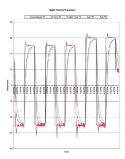
NOTE: While the devices were stable once the temperature was reached there were sporadic connectivity issues during the transition, especially from cold to hot. The devices became stable and responsive once the temperature stabilized and remained constant.
